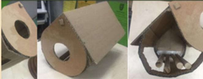
...le of issues with the model, noticeably that the dowels did not run parallel to the front support from the tape, and that the front was an odd shape. Luckily both these were fixed when proper materials are used as the rigidity of the acrylic will mean the front will be the same shape and the glue used to attach the dowel to the back will be much stronger. It is now right with enough space to fit birds or the user's hand without being too hard to open and too much wind.
