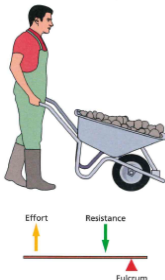
Figure 3 Second-class lever system
